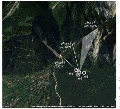
Infrasound radiation by debris flow is highly incoherent, limiting the applicability of xcorr for event detection. Efficiency strongly site dependent.
